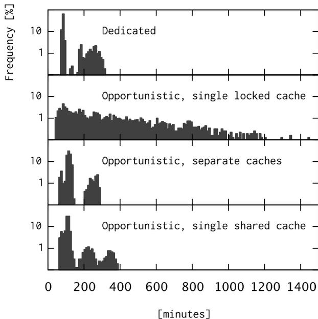
Figure 5. Total job time (aggregate of overhead and processing times)
